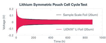
The performance of LIOVIX® based thin foil is similar to extruded, roll pressed thin foil.
