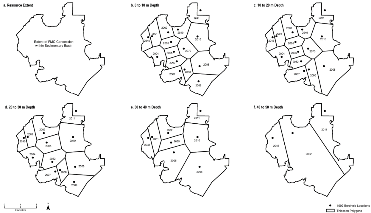
Figure 11-1. Thiessen Polygon Approach to Resource Assessment Using 1992 Exploratory Boreholes
